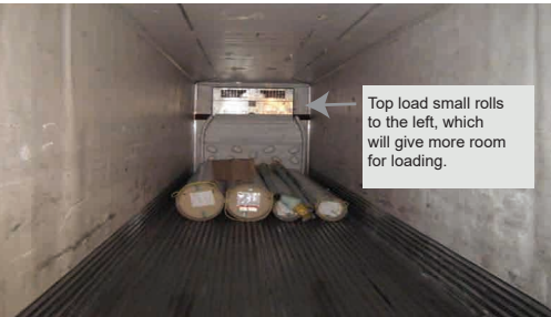
Actual dimensions are 12' feet long. Once small rolls are top loaded to the left, palletized freight can be loaded on right hand side. Cube as 144L x 48W x 96H.
