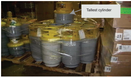
Apply actual dims (dimensional weight) to highest point of freight L x W x H (height of tallest cylinder)
