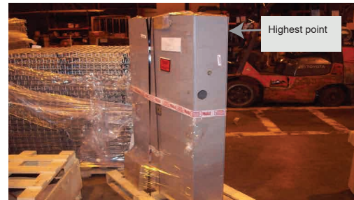
Apply actual dims to highest point of freight L x W x H.
